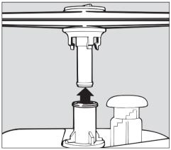
Take off the **lower** spray arm. The lower basket must be removed first.
